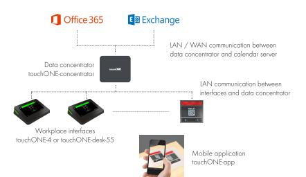
All units are connected to the network. Workplace interfaces communicate with the data concentrator used for system setup as well as for communication with calendar servers. All workplace interfaces are connected using one network cable delivering data and power supply.
